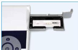
Place the strip inside the Vertu reader (the round opening facing inwards), then press the center key.
