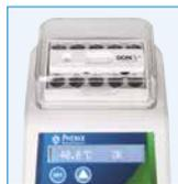
Place DON-V™ strip into the mini-incubator at 40 °C and close the lid. Incubate strip for 2-10 minutes. This can be started while doing the the sample extraction and filtration.
