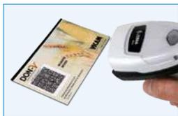
While waiting for 5 min, prepare Vertu calibration by scanning the corresponding barcode for the specific mycotoxin kit.
