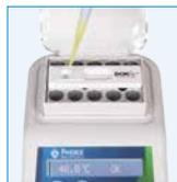
Pipette 100 µL of extract to the sample well on the DON-V strip at 1 drop/second and wait for 5 minutes, leaving it inside the incubator (40 °C).
