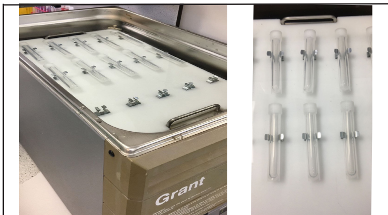
Figure 1. Attachment of 13 mL polypropylene tubes to a polypropylene tube-holder in a Grant OLS 200 water bath.
